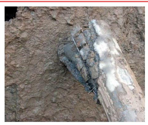
13 Stories, on grade, with no basement, and tied down with hollow pilings with no rebar and significant uneven lateral pressure. The results are no surprise.
